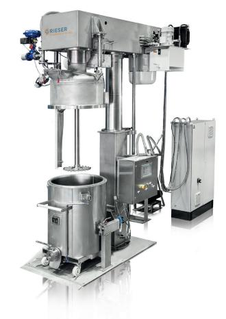
In dispersion, the interaction of mass acceleration and friction forms the basis for the product-specific, ideal shear rate. The proven adjustment of mixing tool, geometry, speed and vessel dimensions produces a highly efficient mixing effect. A large-volume recirculation ensures that the solids are drawn in quickly.
