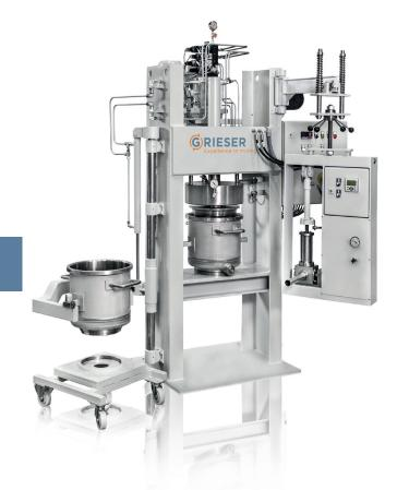
For discharging of highly viscous media, the product is precisely positioned in the squeezing device directly from the mixing container. The press plate contour, which is precisely adapted to the container, enables the containers to be emptied without dead space and with a minimum residual quantity. The design as a vacuum press also guarantees a reliable and bubble-free filling without air pockets in the product.
